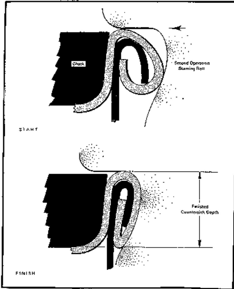
Figure 3.5.c - Second Operation Seam Formation
