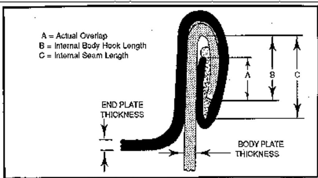
Figure 3.5.2.a - Overlap and Body Hook Butting
