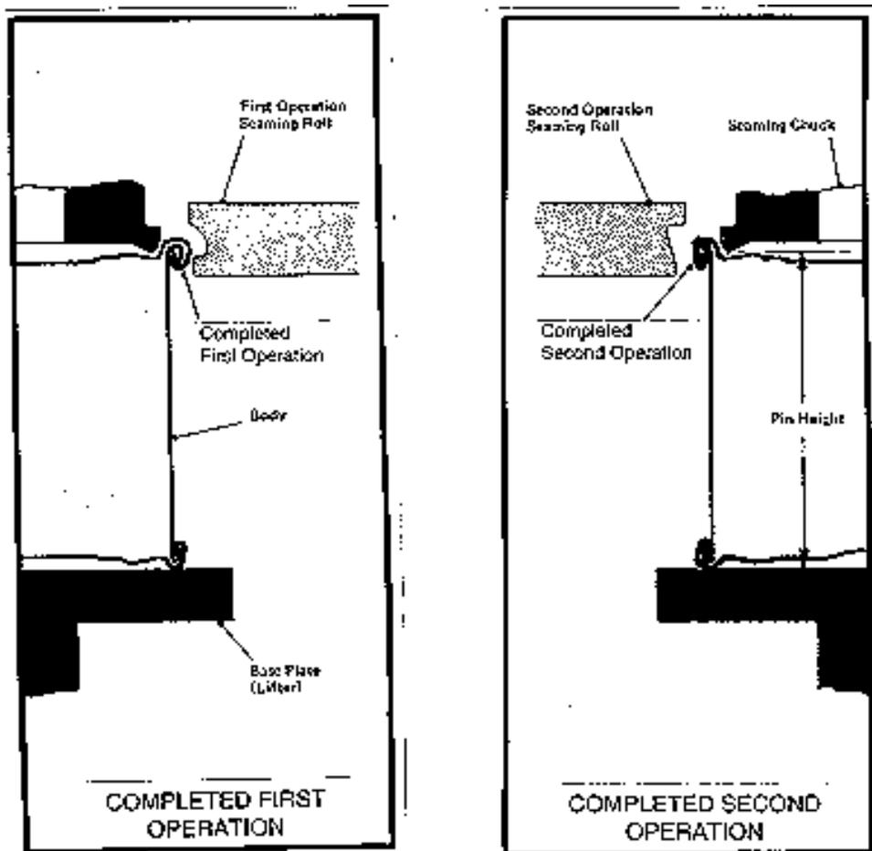
Figure 3.5.a - Basic Double Seamer Design
